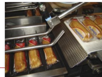
Automation of the individual madeleine production line
